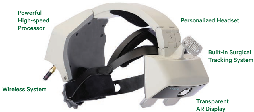
Figure 3. Features Provided by Commercial Augmented Reality Headset. Reprinted with permission from Augmedics, Arlington Heights, Illinois.
