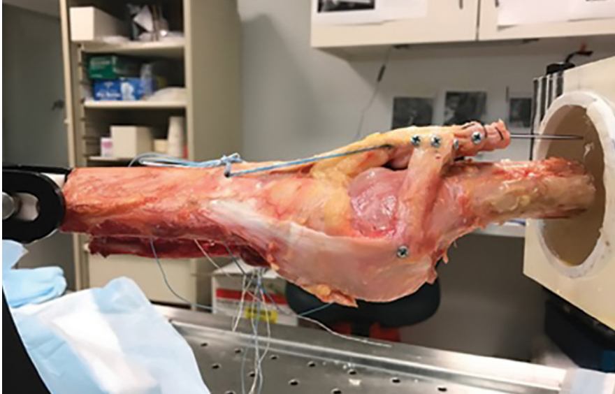
Figure 2. Experimental setup. We potted the knee in PMMA and placed it in a custom-made jig that allowed for 0° to 90° of flexion.
