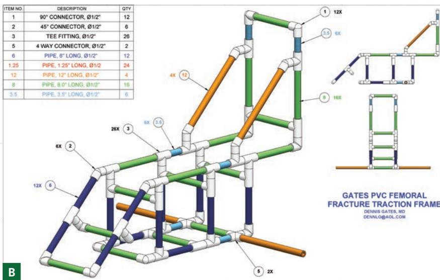
Figure 1. Frame Setup.
