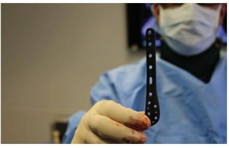
**Figure 1.** Carbon-fiber-reinforced polyetheretherketone anatomic distal fibula plate is shown prior to implantation.
