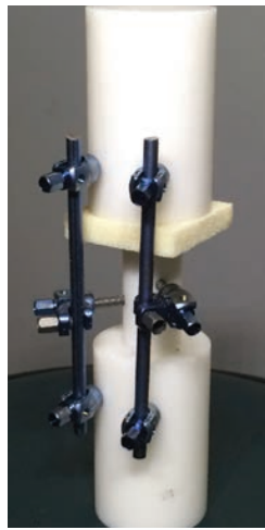
Figure 2. The test state: an idealized spondylectomy model, with Delrin vertebral bodies, posterior segmental screw-and-rod instrumentation, Sawbones cancellous foam at superior endplate, and connected Delrin anterior cage.
