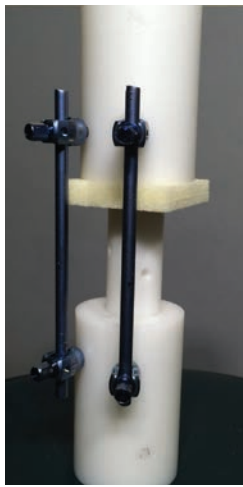
Figure 1. The control: an idealized thoracolumbar spondylectomy model, with Delrin vertebral bodies, posterior segmental screw and rod instrumentation, Sawbones cancellous foam at superior endplate, and a free Delrin anterior cage.
