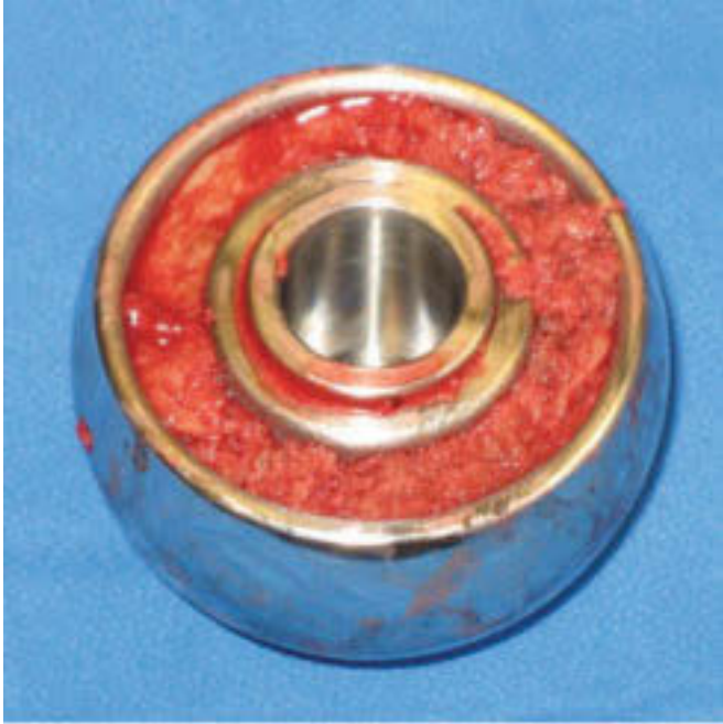
Figure 2. Intraoperative photo from a case outside of the present study showing fretting corrosion at the modular femoral head-neck junction resulting in metallosis and metal ion release.
